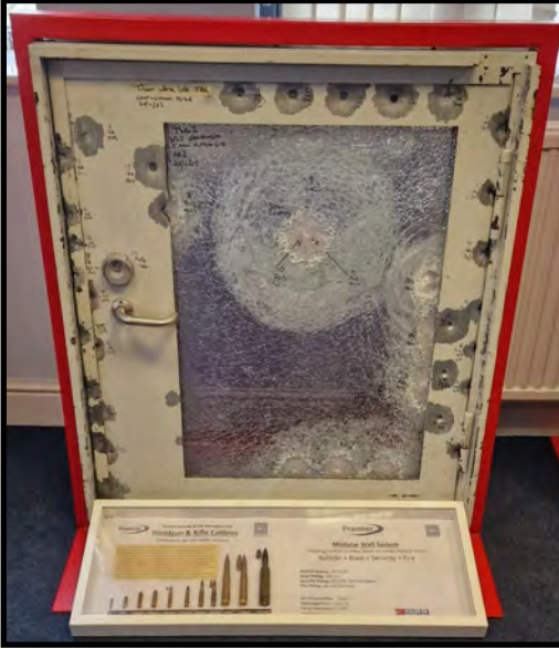
ABOVE: (left) Premier's tested LPS1175 SR3 (C5) security and FB4 Ballistic Glazed system (Right) Premier's tested LPS1175 SR4 (D10) security and FB4 Ballistic Glazed system
