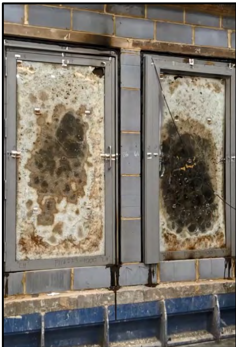
BRE (Building Research Establishment) fire-testing of Premier Security products
