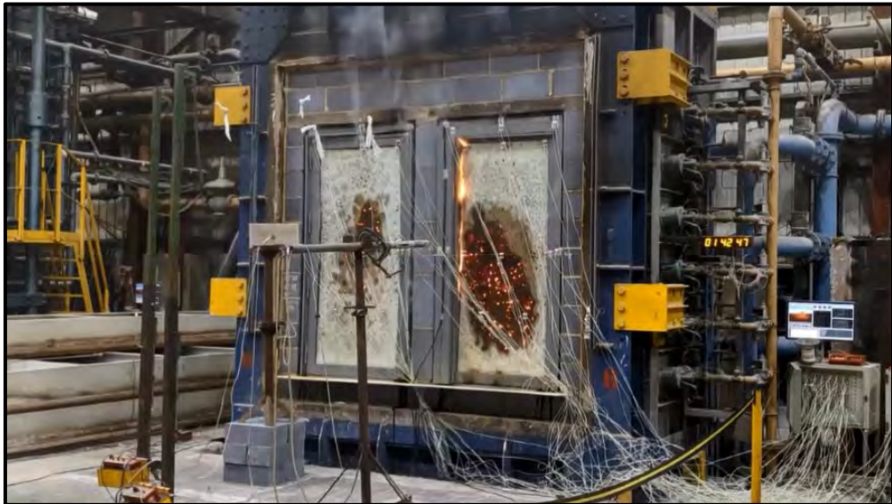
BRE (Building Research Establishment) fire-testing of Premier Security products
